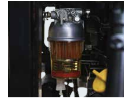
Large fuel / water separator Prevents water/moisture and dust from entering the engine.
