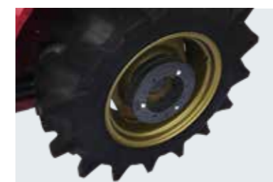
Rear wheel weight (1A8253-34990) Mount any combination of one 20kg, and two 25kg weights for a maximum of 70 kg, on the rear wheels for added traction.
