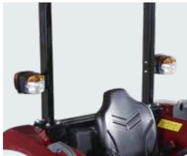
ROPS Yanmar provides ROPS as standard to reduce the chance of injury in the event of tractor roll over.
