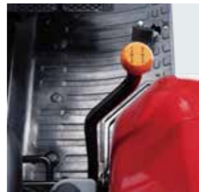
B 4 speed synchronized main shift lever
