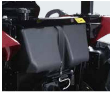
High-capacity fuel tank A capacity of 50 liters lets you work all day without having to stop for refueling.
