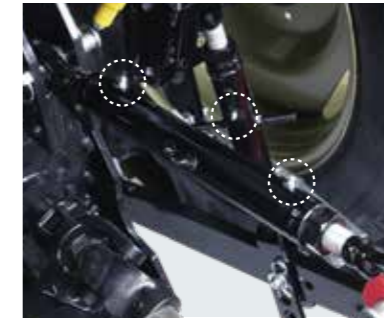
Grease fittings Allocating greasing nipples to appropriate locations. Periodical refilling of grease maintains the life of your machine.
