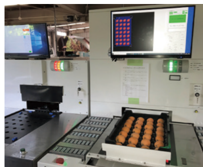
Appearance, weight, and internal quality measurement system for loquats
