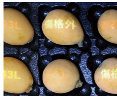
Displaying sorting results by projection mapping
