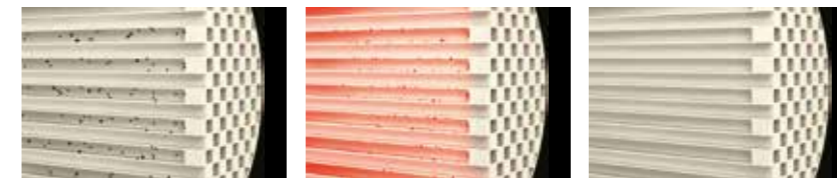
1. Particulate matter trapped 2. Regeneration starts 3. Regeneration completes*
