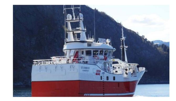
Stormhav is designed and developed by the maritime engineering company Seacon AS in Måløy with design designation SC28. The new vessel has 206 cubic metres of refrigerated/chilled fishroom space, capacity for 90 cubic metres of fuel and accommodation for a crew of up to 14. The vessels of the SC28 series are optimized with regard to regulations, and constructed with a strong focus on design, comfort, environment and catch quality.
