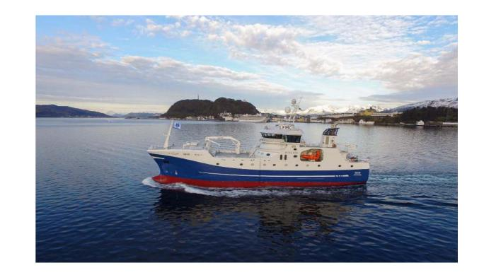
The new Geir is Skipsteknisk's ST-156XL design. The ship is especially designed for longline fishing through a moonpool with a 70,000-hook autoline system. A moonpool is an opening in the base of the hull, giving access to the water below, allowing the crew to work protected from severe weather conditions. The fishing company and designer worked closely together to develop a highly efficient vessel, focusing on environmental footprint, working environment and quality of the final fish product.
