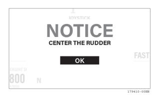
Note: This notice appears when a rudder sensor is not installed. If a rudder sensor is installed, this message appears when the rudder is not centered.
