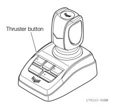
1. When pressing the thruster button, the button flashes, and the notice "THRUSTER MODE STAN-DYBY" appears for 2 seconds together with a buzzer sound. This is the stand-by state.
