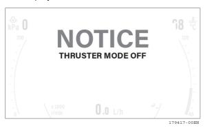
Note: If there is no operation within 10 seconds, stand-by mode is automatically canceled. If there is no operation for 30 minutes in thruster mode, the mode is automatically canceled. At this time, the notice "THRUSTER MODE AUTO RELEASE" appears for 2 seconds accompanied by a buzzer sound and the light turns off.
