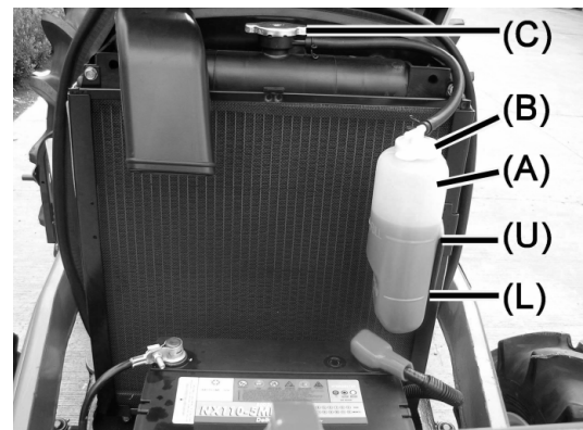
(A) Sub-tank (cooling water) (B) Cooling water supply port (C) Radiator cap (U) Upper limit (FULL) (L) Lower limit (LOW)
