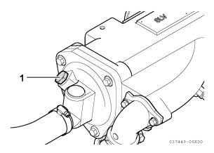
Heat Exchanger Zinc Anode
