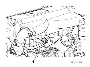
Condensed Water Drain Plug
