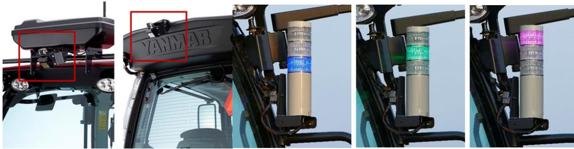
The safety sensor detects people or obstacles (left), and the three-color safety lamp (right)
