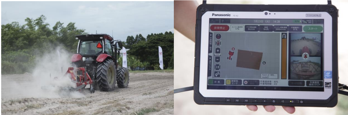
The robot tractor working in the field (left). Control tablet for operation and settings (right).
