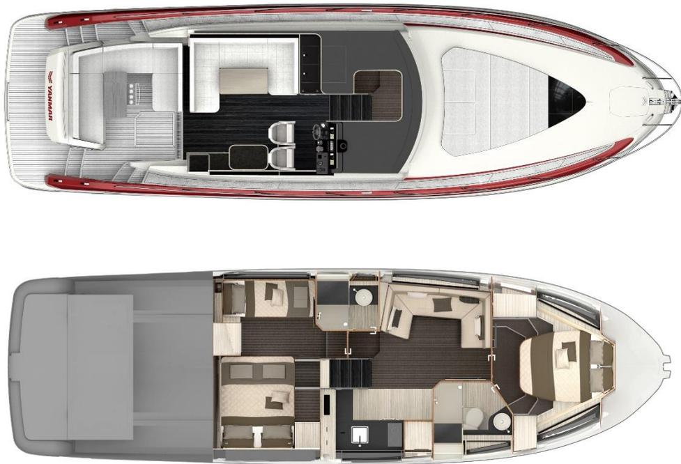
Example of X47 deck layout (top) and interior layout (bottom).
