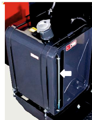
Large-capacity fuel tank (90 L) with fuel indicator
