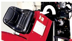
Tilting seat arrangement for easy Engine maintenance
