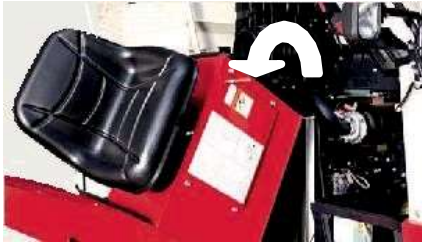
Tilting seat arrangement for easy Engine maintenance
