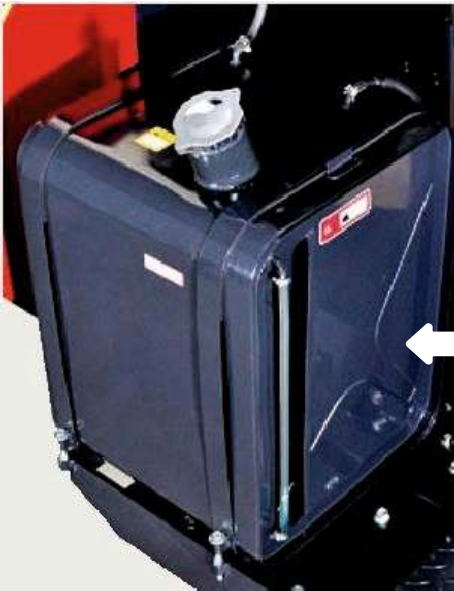
Large-capacity fuel tank (90 L) with fuel indicator
