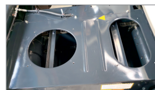
Feeder House, Easy for Assembling and Cleaning
