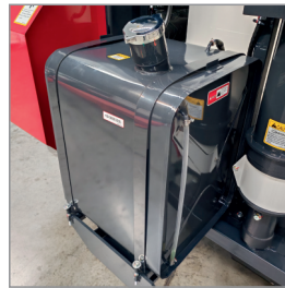
Large-capacity fuel tank (90 L) with fuel indicator
