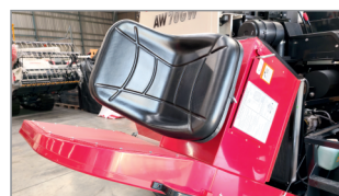
Tilting seat arrangement for easy Engine maintenance
