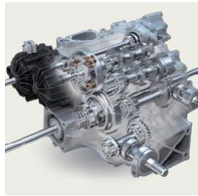
HMT (Hydro-Mechanical Transmission)
