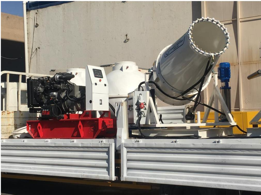
The disinfectant sprayer is powered by a Qaswaa Al-Bararry generator with a Yanmar TNV engine.
