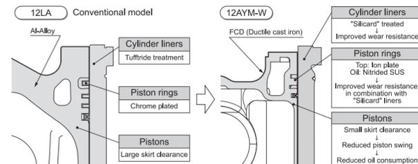
\*\* Sillicard is a surface treatment that uses a special method to embed powdered Silicon Carbide (SiC), an artificial ceramic second only to diamond in hardness, to provide superior wear resistance and durability.
