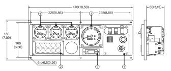
Switch unit (2) Alarm lamp unit (3) Tachometer unit (5) Clock unit Kev switch Alarm buzzer Alarm buzzer stop switch Stop button
