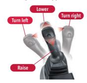
To prevent malfunctions, the operator must press the vessel lock release switch to raise or lower the vessel.
