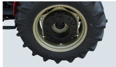
Rear wheel weights (Including left and right sides) Base weights 40kgx2 (1A8263-91210) Additional weights 40kgx4 (1A8296-91220) Base & Additional weights 40kgx2 & 40kgx4 (1A8263-91200) Weights can be attached to the rear wheels on one side up to 120 kg to increase traction.
