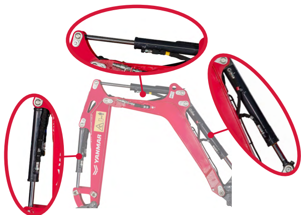
Cylinders mounted over the boom
