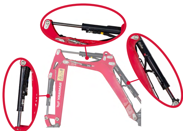
Cylinders mounted over the boom
