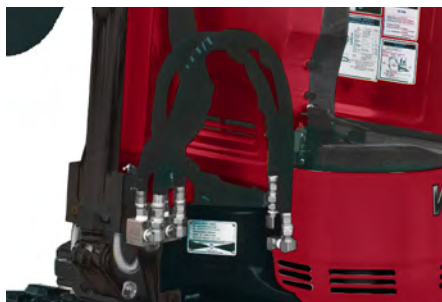
2 Careful routing of hydraulic pipes and hoses.
