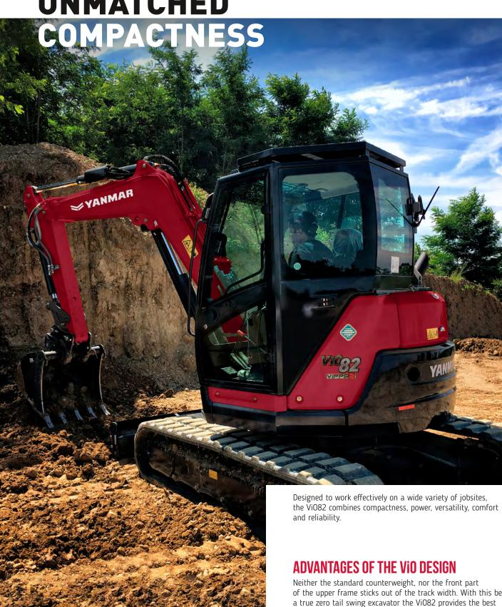
of the upper frame sticks out of the track width. With this being a true zero tail swing excavator the ViO82 provides the best conditions for working safely and comfortable on any working site with limited space.
