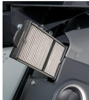
Even the air filters have been located in easy-to-access spaces, to ensure quick and simple maintenance.
