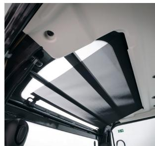
The roof window of the SV60-6B is protected by a fully integrated sunshade for a maximum comfort.
