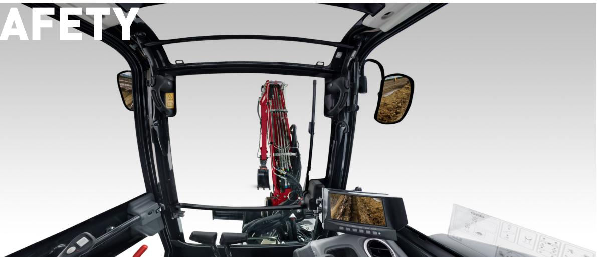
The SV60-6B cab has been designed to meet ROPS (Roll-Over Protective Structure) certification, as well as FOPS (Falling Object Protective Structure) level 1. The cab can be fitted with FOPS level 2 protection (front and top guard) as an optional extra.
