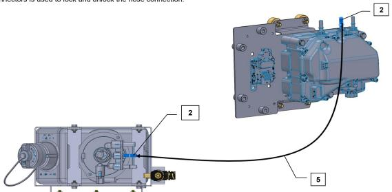
12 Attach the Hose, 3/8" ID, Supply Line (4) to the Supply Module (30) and the DEF Tank (2). A white ring on each Hose (6)
