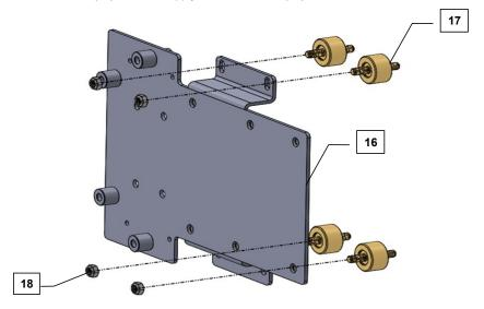
8 Install Nox modules (31) to the Supply Module Bracket (16) as shown in the picture below using Bolt, M8-1.25X16 (13) and Nut, M8 (14).
