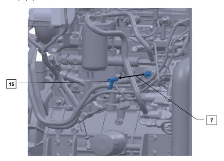
14 Cut the Hose, 3/8" ID (8) provided in the DEF kit to precise length - 29.5", and attach it to the Tee Fitting (15) and the Dosing Module (32) using Hose Clamps (12).
