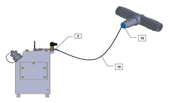
16 Cut the Hose, 1/2" ID (9) provided in the DEF kit to precise length - 70.8", and attach it to the DEF Tank (2) and the Engine water pump inlet using Hose Clamps (12).
