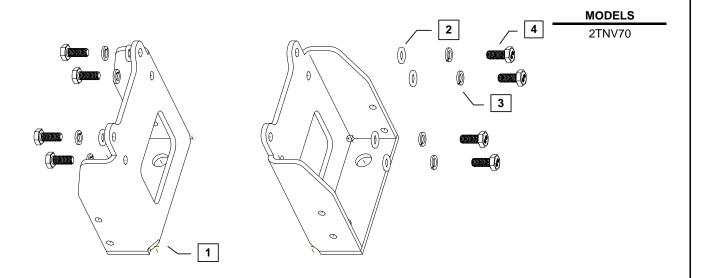
Remarks: (A) 26106-100202 is a service part used to replace the bolt, lock washer and washer assembly (items: 2, 3 and 4).
