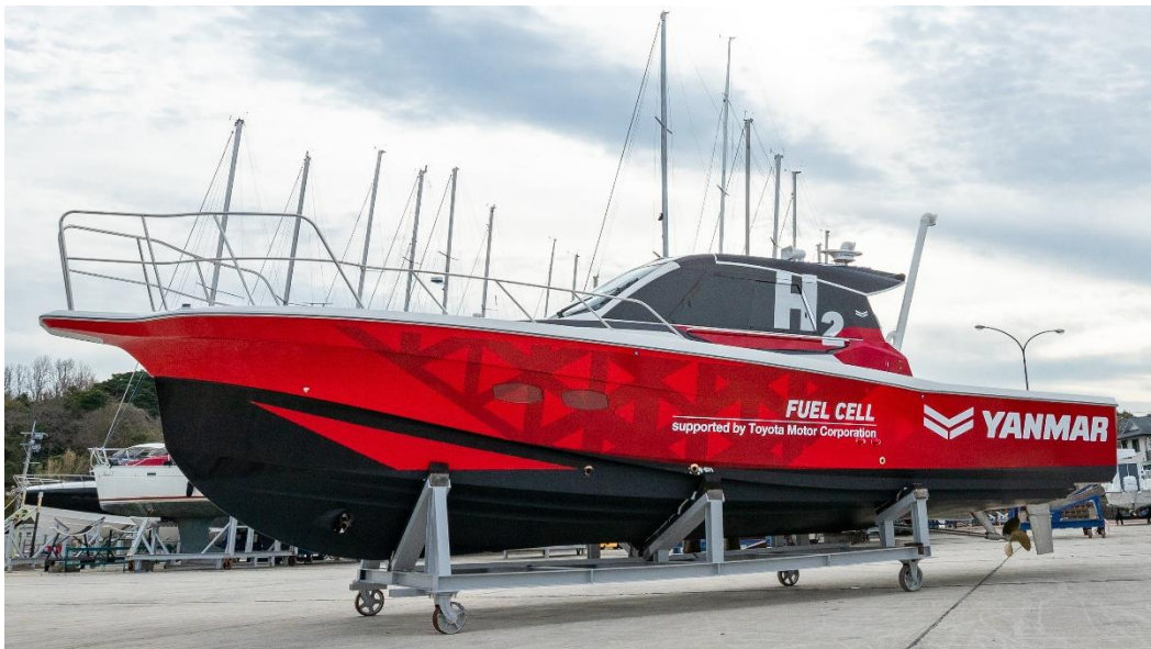
Demonstration test boat with maritime fuel cell system
