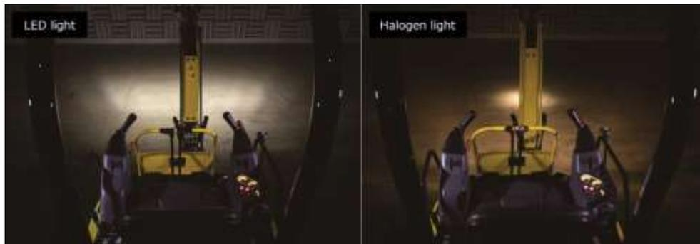
Comparison of LED light and halogen light illumination
