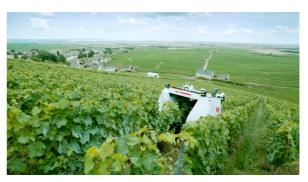
Using an advanced spraying system, YV01 ensures that vines are precisely sprayed with the exact amount of droplets which means less spraying fluids are required.
