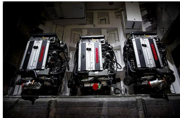
Left: interior design of the X47; right: triple arrangement of 8LV marine diesel engines.
