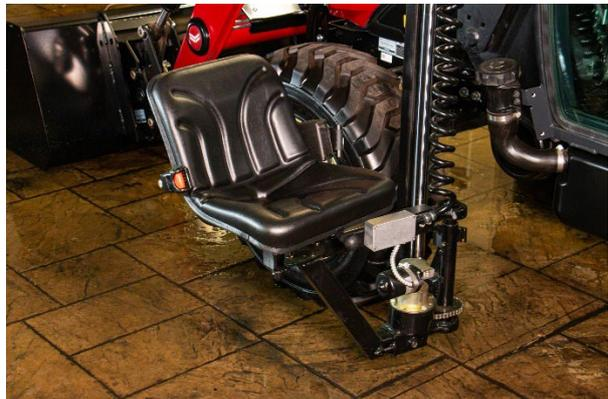
Left: The Yanmar YT3 can be easily fitted with hand controls; right: a chair lift transfers the user to the cabin.
