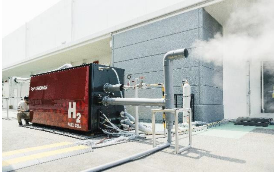
Left: Test scene of the marine hydrogen fuel cell system*1; right: Image of installation into a ship
