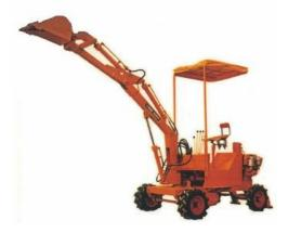
had a sliding boom that allowed it to excavate right up against walls. By 1974 Yanmar miniexcavators were fitted with cabins, and noise suppressed to allow them to work in confined spaces, residential areas, and at night.
