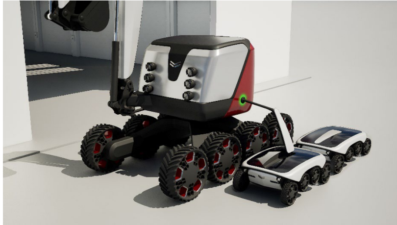
Image of a self-propelled battery vehicle automatically supplying power to electric construction equipment.
