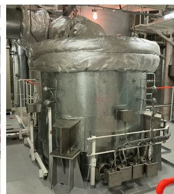
[Methane slip reduction system on board (Left: EGR Note2 system, Right: Methane oxidation catalyst layer)]
