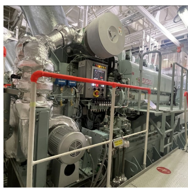
[Methane slip reduction system on board (Left: EGR Note2 system, Right: Methane oxidation catalyst layer)]
