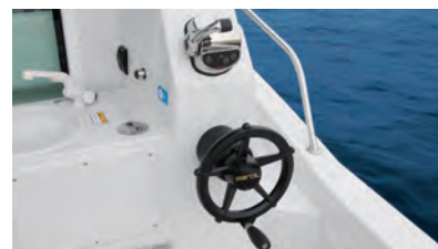
Aft deck steering station
