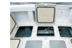
Storage/propeller & steering inspection compartment
