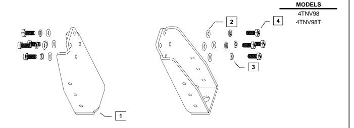
Remarks: (A) 26106-100202 is a service part used to replace the bolt, lock washer and washer assembly (items: 2, 3 and 4).
