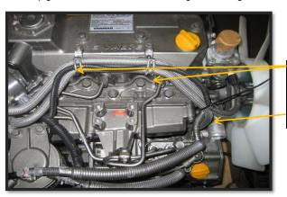
Coolant sensor wire routed through the EGR coolant clips. The coolant hoses and harness are secured with a wire tire close to the thermostat.
