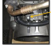
HellermanTyton mount and large wire tie to hold down the large section of loom to the flywheel housing. Make sure mount and loom have the proper orientation to allow the loom to rest close to the flywheel barrel.
